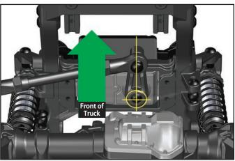
If you are using aftermarket servos, it is important to use servo horns designed for TRX-4 Sport. The servo horns must measure 22mm from the steering linkage mounting hole to the servo mounting hole.
