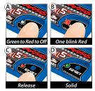
The LED will blink and then turn solid green (Low-Voltage Detection ACTIVE) or red (Low-Voltage Detection DISABLED). The model is ready to drive.
