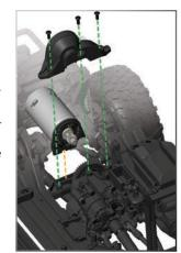
motor pinion (9-T - 22-T) and spur gear size (39-T or 45-T). Remove the two screws from the motor/motor plate and reinstall in the corresponding positions; reinstall the motor/motor plate assembly in the chassis.
