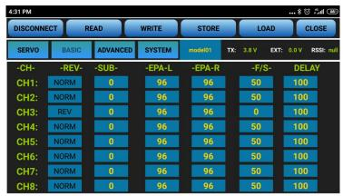
**REV:** Defines the relationship between the transmitter controls and the receiver output for channels with options of NORM and REV. Make sure to check all servos move to the correct direction as wish under control. Make sure to check all servos move to the correct direction under control.
