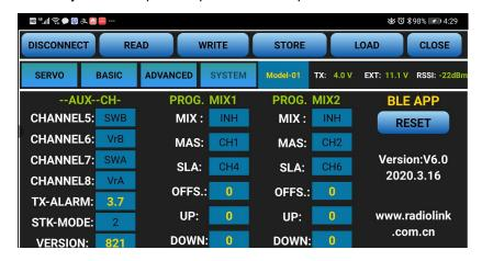
(DIS)CONNECT: When APP is opened on the mobile and T8S is powered on, click CONNECT and a list of Bluetooth devices will pop out and select the RadioLink device to make connection. If not succeed, click DISCONNECT then make sure the APP is closed at the back stage then CONNECT again. Every time open the APP, the data displayed are the ones last time disconnected.
