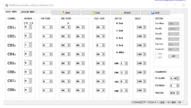
**REVERSE:** Defines the relationship between the transmitter controls and the receiver output for channels with option of NORM and REV. Refer to 3.3.2-**REV** (P8) for more details.
