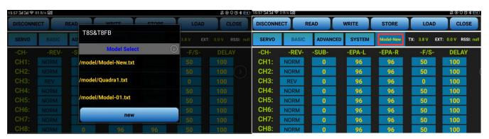
There are four parameter setup menus: SERVO/BASIC/ADVANCED/SYSTEM
