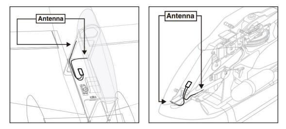
\*The two antennas should be placed at 90 degrees to each other.
