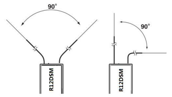
This is not a critical figure, but the most important thing is to keep the antennas away from each other as much as possible.
