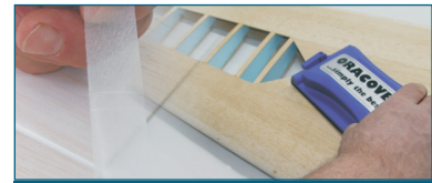
Fig. 2: Smooth sanding of the structural surface
