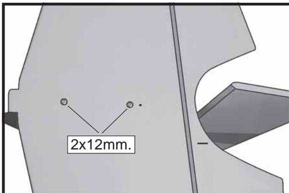
□ 3) Slide the set of vertical and horizontal tail fin to the fuselage.
