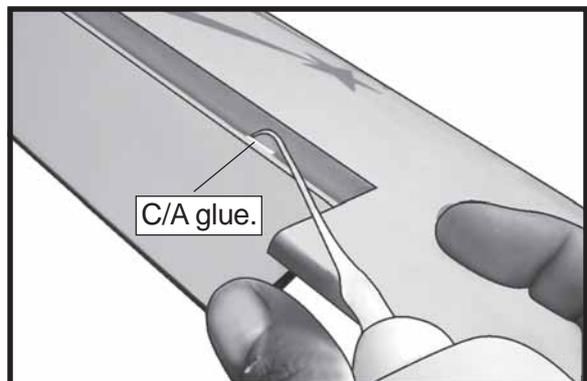
□ 5) Turn the wing panel over and deflect the aileron in the opposite direction from the opposite side. Apply thin C/A glue to each hinge, making sure that the C/A penetrates into both the aileron and wing panel.
