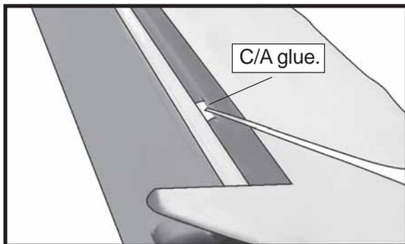
□ 6) Using C/A remover/debonder and a paper towel, remove any excess C/A glue that may have accumulated on the wing or in the aileron hinge area.
