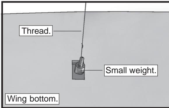
Attach the thread to the servo lead and carefully thread it through the wing.
