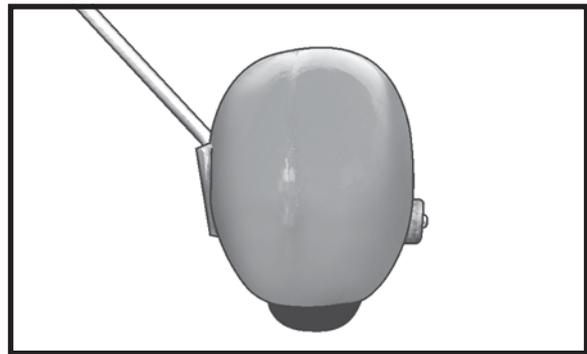
A drop of C/A glue on the wheel collar screws will help keep them from coming loose during operation.
