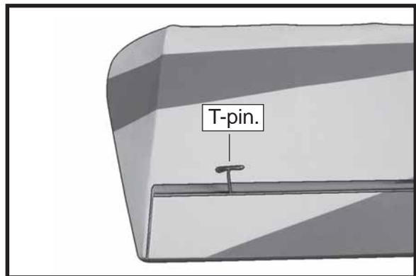
□ 4) Deflect the aileron and completely saturate each hinge with thin C/A glue. The ailerons front surface should lightly contact the wing during this procedure. Ideally, when the hinges are glued in place, a 1/64" gap or less will be maintained throughout the length of the aileron to the wing panel hinge line.
