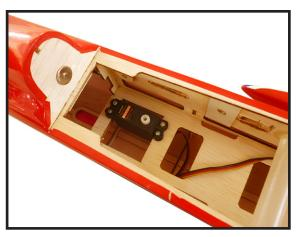
5) Insert the Z-bend from the pushrod wire through the hole in the servo horn.
