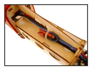
5) Route the battery lead through the opening in the fuselage. The lead for the receiver is routed under the battery tray and receiver, then plugged into the throttle channel of the receiver. Mount the switch from the speed control in the fuselage where it can be accessed when the canopy is removed.
