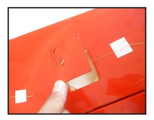
2) Place the servo between the tabs on the servo cover with the output of the servo over the opening in the cover. With the servo spaced slightly off the cover, use a pencil to mark the location for the servo mounting screws.
