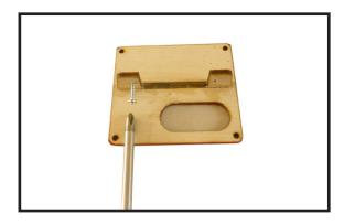
5) Apply 2-3 drops of thin CA in each of the holes to harden the surrounding wood. This will harden the threads so the screws do not easily strip the surrounding wood.
