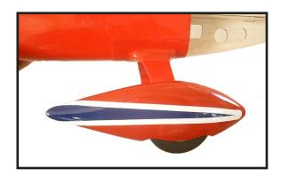
4) Repeat above steps to install the remaining wheel and wheel pant on the landing gear.
