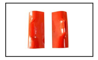
6) Fit the landing gear fairings over the gear. Slowly trim the fairing to fit to the fuselage. When installed, they will cover the area where the landing gear attaches to the fuslage.
