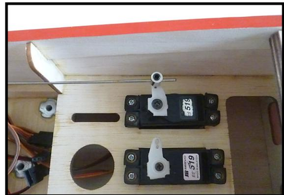
9) Move the throttle stick to the closed position and move the carburetor to closed. Use a 2.5mm hex wrench to tighten the screw that secures the throttle pushrod wire. Make sure to use threadlock on the screw so it does not vibrate loose.
