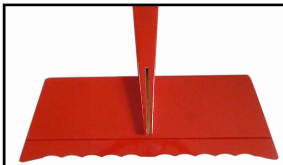
4) With the stabilizer held firmly in place, use a pen and draw lines onto the stabilizer where it and the fuselage sides meet.
