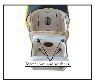
4) Attach the motor to the front of the electric motor box using four 4mm blind nut, four M4x20mm hex head bolts to secure the motor. Please see picture shown.
