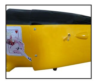
Because of the size of the cowl, it may be necessary to use a needle valve extension for the high speed needle valve. Make this out of sufficient length 1.5mm wire and install it into the end of the needle valve. Secure the wire in place by tightening the set screw in the side of the needle valve.
