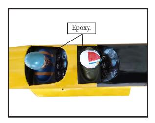
4) Epoxy canopy onto the fuselage. Trace around the canopy and onto the fuselage using a epoxy.
