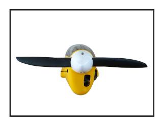
The propeller should not touch any part of the spinner cone. If it does, use a sharp modeling knife and carefully trim away the spinner cone where the propeller comes in contact with it.
