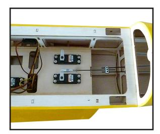
RUDDER PUSHROD HORN INSTALLATION.
