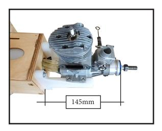
2) Use a pin drill and 4mm drill bit to drill a small indentation in the mount for the engine mounting screw.
