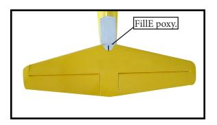
□ 2) Slide the vertical stabilizer back in place. Using a triangle, check to ensure that the vertical stabilizer is aligned 90° to the horizontal stabilizer.
