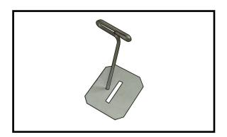
2) Remove each hinge from the wing panel and aileron and place a T-pin in the center of each hinge. Slide each hinge into the wing panel until the T-pin is snug against the wing panel. This will help ensure an equal amount of hinge is on either side of the hinge line when the aileron is mounted to the aileron.
