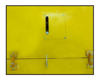
INSTALLING THE FLAP PUSHROD.
