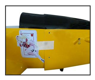
2) Use a drill and drill bit to drill the holes for the cowl mounting screws. Make sure the cowl position is correct before drilling each hole.
