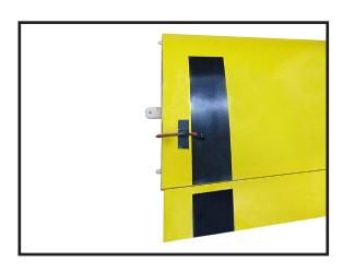
8) Set the aileron hatch in place and use a Phillips screw driver to install it with four wood screws.
