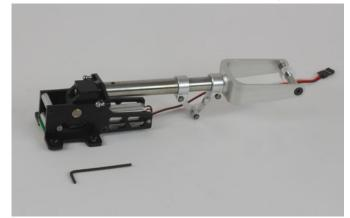
Includes one (1) Aircraft Mechanics 25-46 size 90° electric retract nose unit, sprung oleo strut, wheel axle, wheel spacers and hex wrenches.
